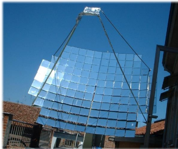
A mirror based photovoltaic concentrator (Courtesy of Univ. of Ferrara, Italy)
